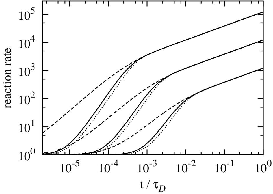
**Figure 3.** Global reaction rates for (solid) Gaussian distributed, (dashed) power-law ( $\beta = 3/2$ ) distributed shear rates and (dotted) constant shear rate for (top to bottom)  $\langle |\sigma| \rangle = 10^2, 10^1$  and 1. The reaction rates are normalized by  $Ls_0\Delta u_0\mathcal{A}/\tau_D$ .
