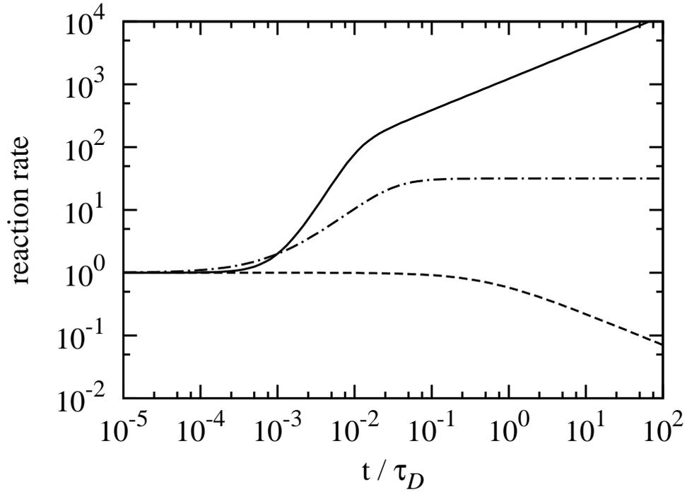
**Figure 2.** Global reaction rates for (solid) linear shear flow with  $\sigma = 1$ , (dashed-dotted) radial flow with  $\alpha = 1$ , and (dashed) uniform flow. The reaction rates are normalized by  $Ls_0\Delta u_0\mathcal{A}/\tau_D$ .
