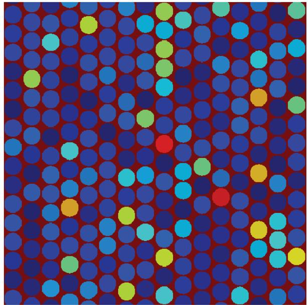
FIG. 1. Illustration of the model medium consisting of a conductive matrix with  $k_0 = 1$  and less conductive disc-shaped inclusions of radius  $r_0 = 1$  and conductivity  $k$ , which is distributed according to  $p_k(k)$ . The inclusions are embedded in a rectangular unit cell of size  $\ell_0$ . Different colors denote different conductivity values.
